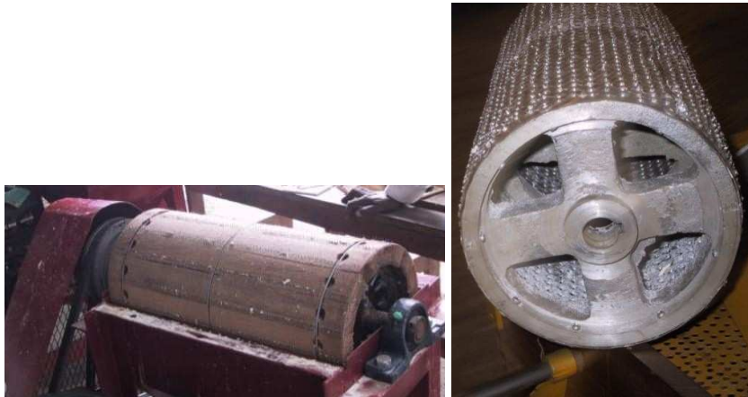
Figure 2: The original wooden drum with spikes and the new metal drum.
