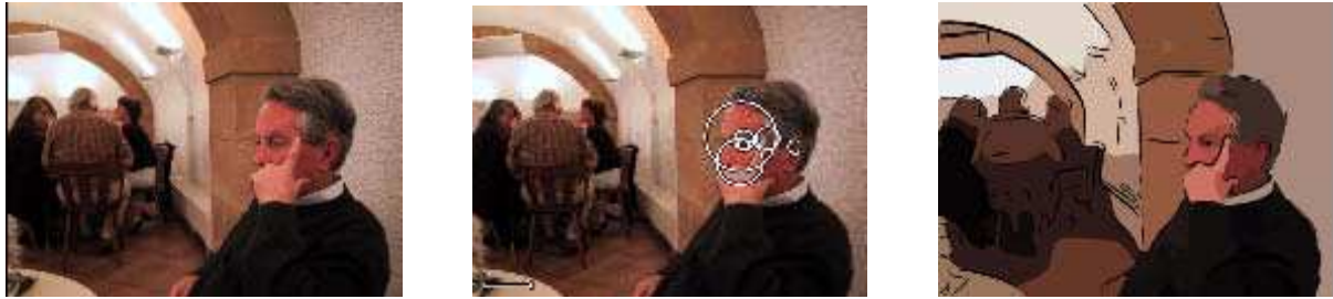
Figure 5: (a) source image; b) fixation points gathered by eye-tracker; (c) the resulting line drawing
