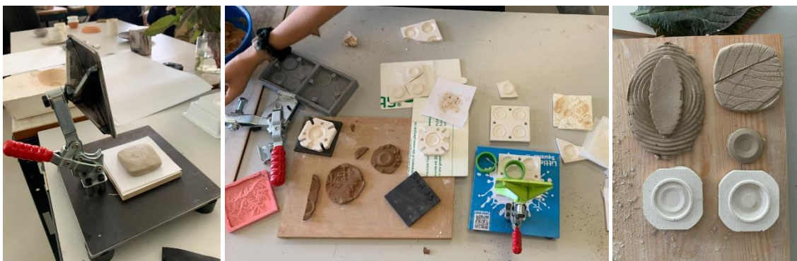
Figure 8: Press-forming clay with small countertop toggle press 'Little Squisher', image by Author 2023
