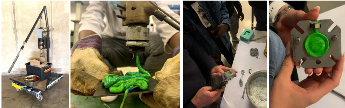
Figure 8: In-class injection moulding. Image by author 2023
